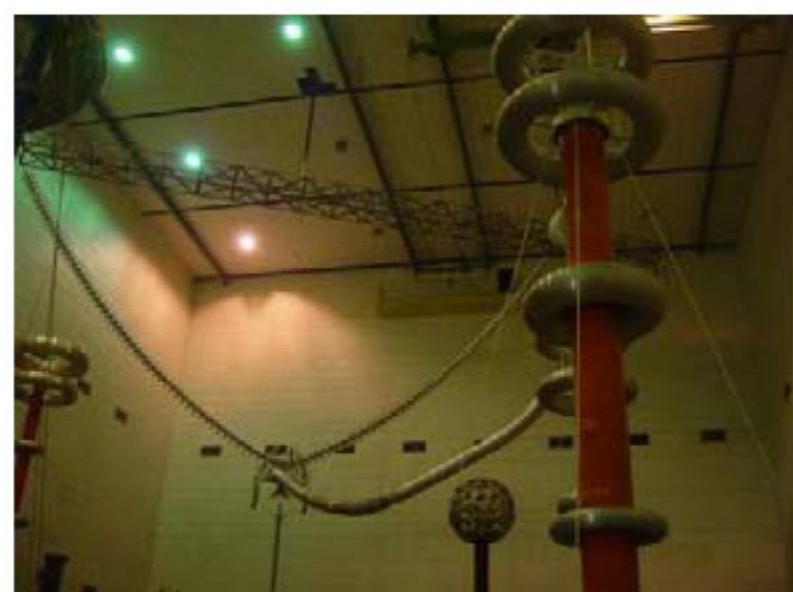
图 10 电压分布测量试验布置 Fig. 10 Test layout of voltage distribution measurement
